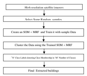
Fig. 2. System Sketch: Image Segmentation Steps of SOFM and MRF
